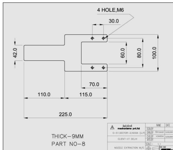
Fig 10: Cantilever support for clamp
