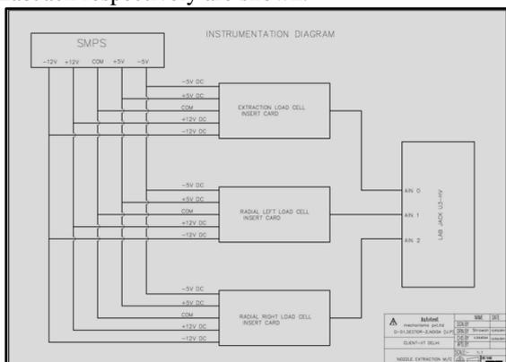
Fig 22: Complete electrical interface diagram
