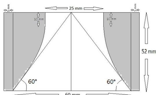
Fig 16: Nozzle with 25 mm top diameter
