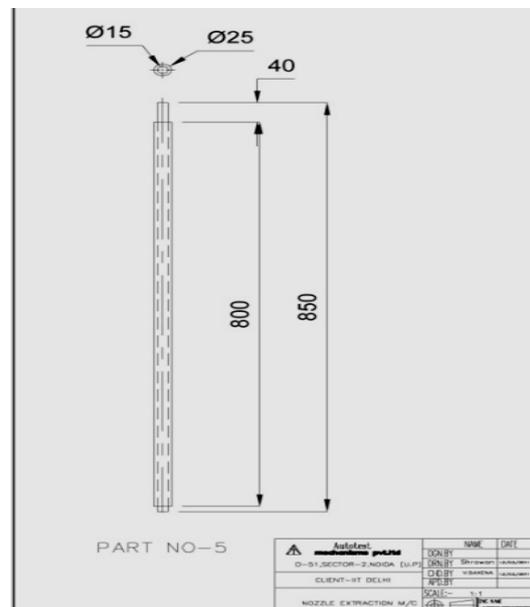
Fig 7: Threaded bar on which movable fabric holder mounted
