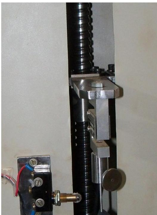
Fig 14: Load cell attached to clamp
