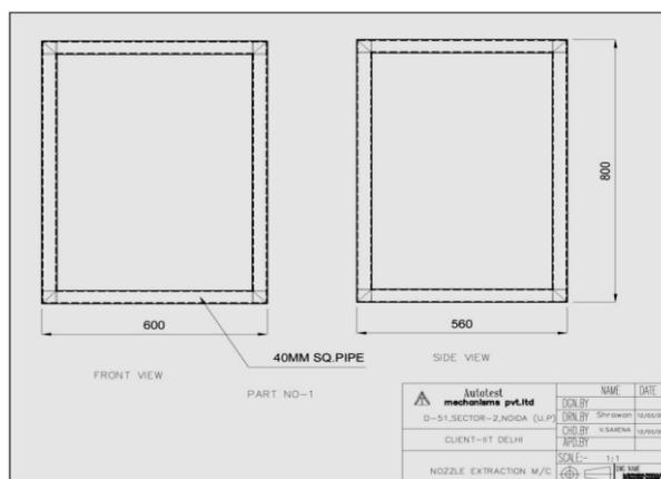
Fig 2: Base cabinet of the instrument
