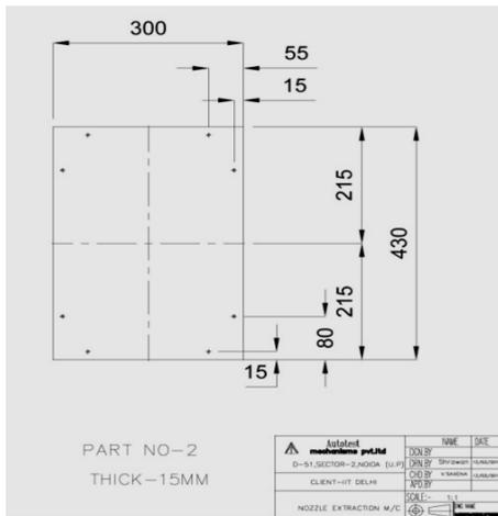
Fig 3: Load cell support base dimensions
