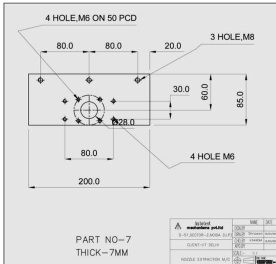
Fig 9: Clamp holder support bolt dimensions and positions
