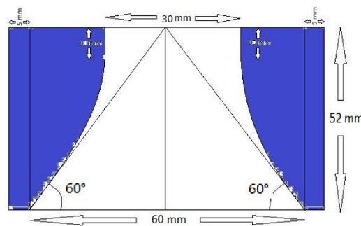
Fig 17: Nozzle with 30 mm top diameter
