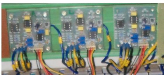
Fig 28: Analog to digital card interface with LabJack
