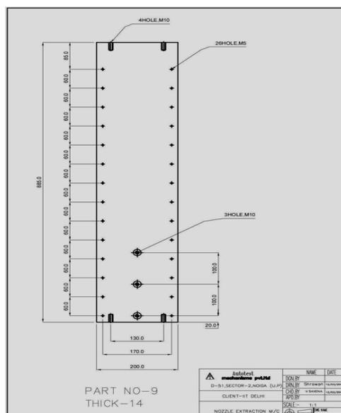
Fig 11: Side support of moving clamp
