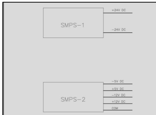
Fig 24: Electrical diagram for SMPS power input/output
