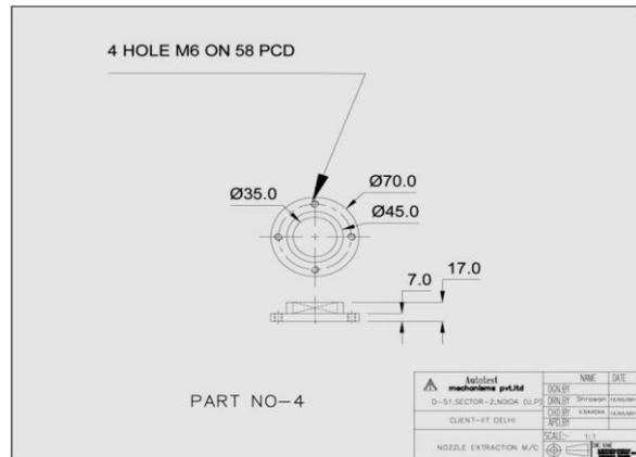
Fig 6: Vertical threaded bar stand base bolt dimensions
