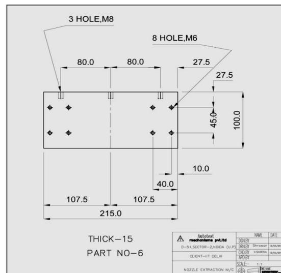
Fig 8: Clamp holder mounting dimensions
