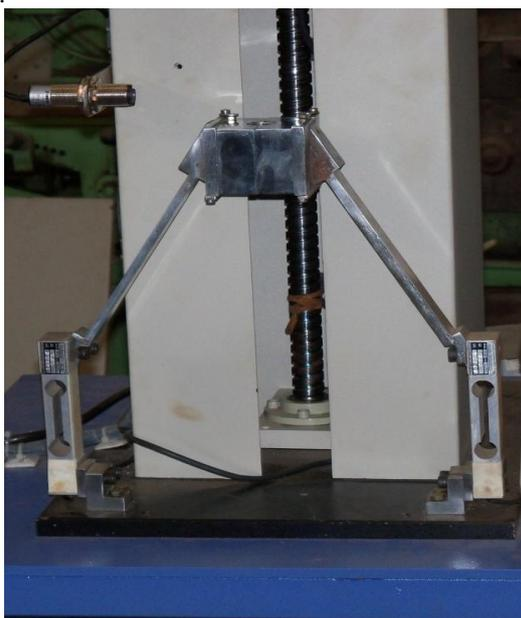
Fig 19: Radial load cell
