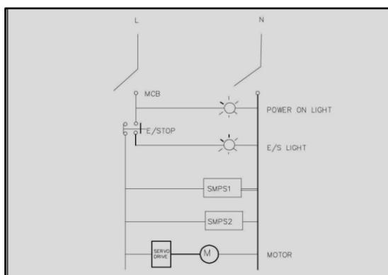
Fig 25: Electrical diagram for power system
