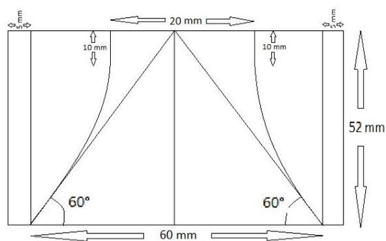
Fig 15: Nozzle with 20 mm top diameter
