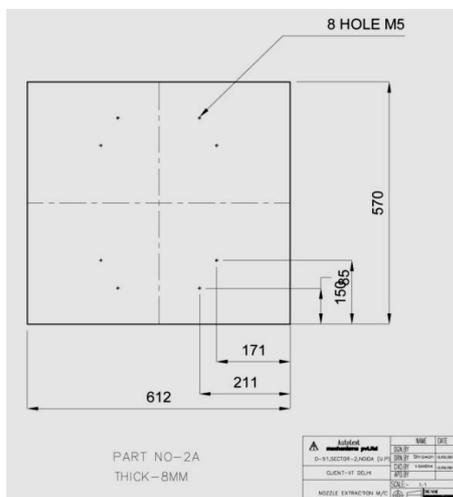
Fig 4 : Cabinet top and vertical stand base dimensions
